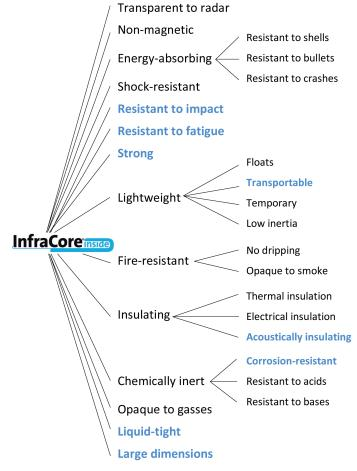
Overview of the properties of InfraCore<sup>®</sup> Inside, with those applicable to civil engineering structures highlighted
