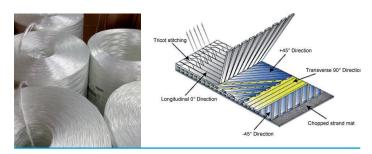
Rolls of glass fibres and an example of a glass fibre fabric comprising multiple fibre directions.
