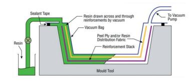
Schematic view of the vacuum infusion technique.
