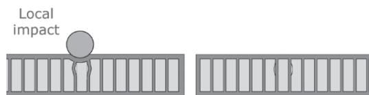
In InfraCore® Inside, local damage can not lead to catastrophic failure modes. Moreover, the core-material (foam) is not part of the load-bearing structure, but only acts as a placeholder during construction.
